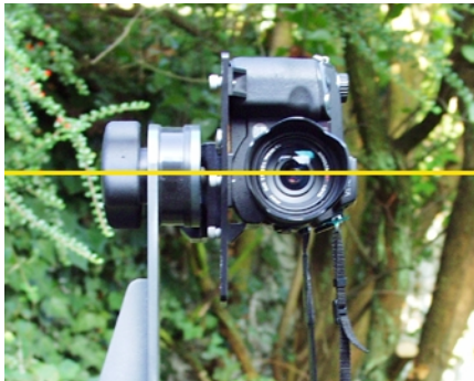
The centre of the lens and the tilting axis are on a same horizontal line.
